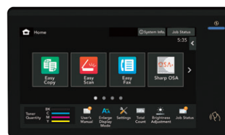
10.1" (diagonally measured) customizable touchscreen display.
