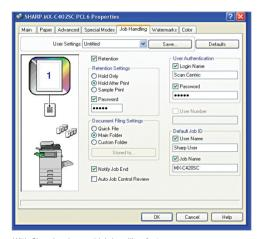
With Sharp's advanced job handling features, users can easily retain print jobs on the MX-C402SC and MX-B402SC hard drives for reprinting at a later date.
