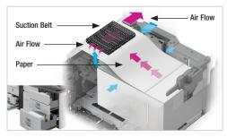
Triple air-feed LCT paper trays maximize reliability and minimize downtime. Pneumatic sensors maintain consistent air flow.
