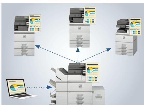
With Serverless Print Release you can securely print a job and release it from up to six supported models (including host).
